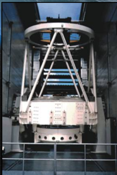
The "Galileo" National Telescope (TNG) is 3.58m Alt-Az telescope equipped with an active optics system. Its two Nasmyth foci host 5 instruments that are permanently mounted and operating.
